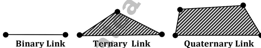
Links can be classified into binary, ternary and quaternary depending upon their ends on which revolute or turning pairs can be placed. The links shown in figures given above are rigid links and there is no relative motion between the joints within the link.
