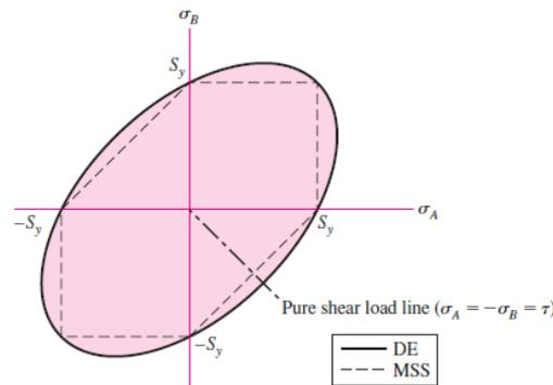
**Fig. 6.1.1 The distortion-energy (DE) theory for plane stress states**
